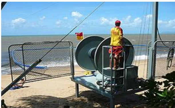
The Uninet Enclosure System, winch on beach
